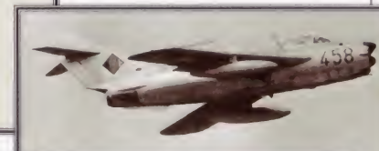
▼ Afterburning night-fighter East Germany operated the radar-equipped, afterburning MiG-17PF 'Fresco-D' all-weather/night fighter.
